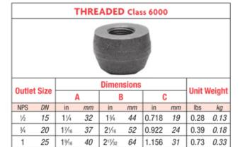
Each outlet size listed is available to fit any run curvature. Threaded ends are in accordance with ANSI/ASME B1.20.1. Design per MSS-SP-97.
