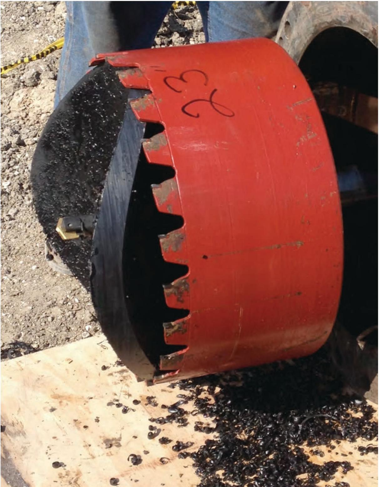
**CUTTING HDPE IS PERFORMED WITH SHARP AND FLUTED CUTTERS. THE PILOT DRILL PERFORMS THE RETENTION OF THE CUT SECTION OR "COUPON" ALLOWING IT TO BE REMOVED UNDER PRESSURE..**
